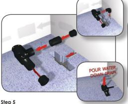
Note: All solvent joints should be cleaned with an appropriate solvent weld cleaner prior to using solvent adhesive.
