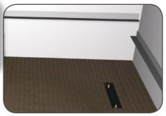
**Step 8**From a roll of waterproofing tape cut to suit the width of the shower tray and the length of the shower tray.
